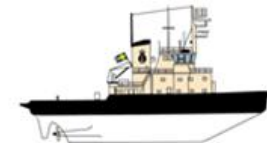
ALE Displ ton 1500 Built 1973 Length 47m Breath 13m 3500 kW
