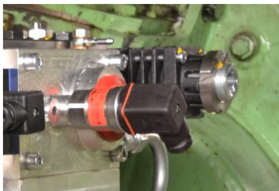
Picture 13: Fuel pressure sensor at K4 pump
