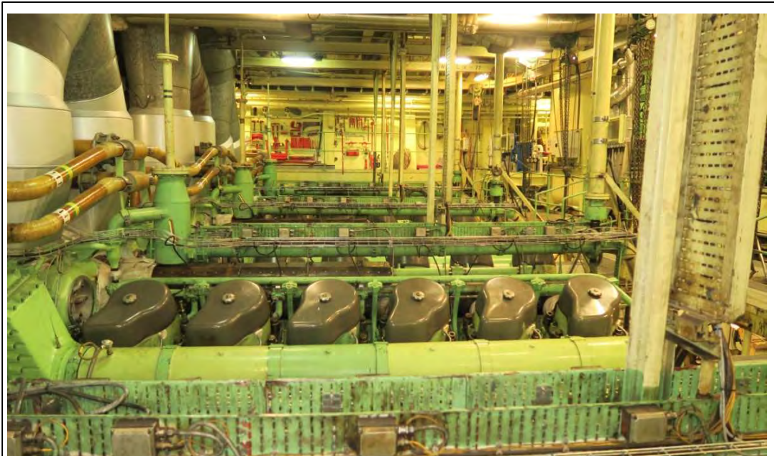
Picture 1: View into the engine room; Overview main engines Pielstick PC 2-2 (V12)
